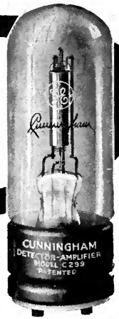
C-299—3 Volts .06 amp. Dry Battery Det. and Amp.
